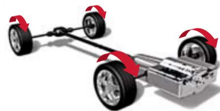
**Continuous AWD** Models equipped with the 5-speed manual use a viscous-center locking differential. Should wheel slippage occur, it helps transfer power to the wheels with the most traction.
