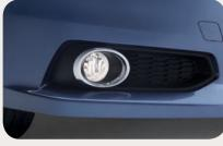
Fog Lights Cast a low and wide beam of light to enhance vision in inclement weather.
