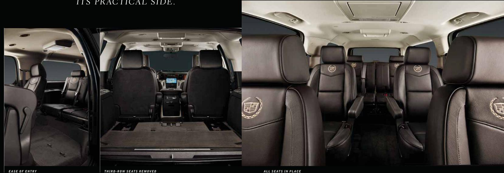
The simple touch of a button sends the second row into motion, folding the seats forward, making it easier for rear passengers to enter.
