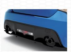
Rear Diffuser. Lower rear body panel helps to direct air flow and adds a sculpted finishing touch to the BRZ lower rear body line.
