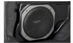
**10-Inch Powered Subwoofer.** The 10-inch powered subwoofer provides powerful deep bass and clean. sound reproduction with its integrated 100W amplifier and a passive crossover network. Manufactured for Subaru by Kicker.<sup>®</sup>
