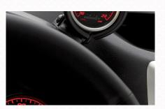
**Turbo Boost Gauge.** Displays engine vacuum in inches of Hg and boost in PSI. Bright red illumination matches vehicle instrument panel lighting and goes dark when the engine is turned off. Includes mounting cup and bracket.
