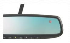
Auto-dimming Mirror with HomeLink.® Mirror darkens when headlights are detected from behind the vehicle. Includes a compass and three integrated HomeLink® buttons that are programmable for most garage-door openers and other HomeLink®-compatible devices.
