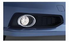
Fog Lights. Cast a low and wide beam of light to enhance vision in inclement weather.
