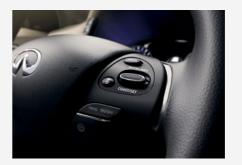
EASE IN TRAFFIC Intelligent Cruise Control (Full-Speed Range)<sup>2,10</sup> allows you to choose your desired speed and following distance, and automatically adjusts your speed in slowing traffic, going all the way to a complete stop. This visionary feature and the personalized convenience it offers is available with a simple touch of a button.
