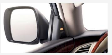
MAINTAINING YOUR LANE The Lane Departure Prevention System<sup>1,5</sup> uses a camera to watch for departure from the traveling lane when you haven't signaled, and audibly warns you if it's detected. Then, if the drift continues, the system lightly applies selected brakes help to ease your vehicle back into the travel lane. But you never give up control. It's designed to assist, not override.
