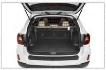
Compartment Separator. Helps to separate cargo from the passenger area.
