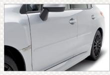
Body Side Moldings. Color-matched moldings help protect the vehicle's doors from parking lot dings while attractively blending with the lines of the car.
