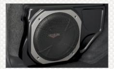
10-inch Powered Subwoofer. The 10-inch powered subwoofer provides powerful deep bass and clean sound reproduction with its integrated 100W amplifier and a passive crossover network. Manufactured for Subaru by Kicker®.
