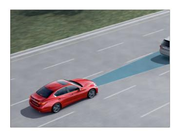
RECOGNIZING DANGER Forward Collision Warning<sup>1,13</sup> looks ahead and if your distance to the vehicle in front is too close, it can warn you visually and audibly.
