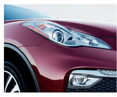
INTUITIVE FRONT LIGHTING Illuminate where you truly want to be. The Adaptive Front lighting System (AFS) with auto-leveling headlights improves visibility at intersections and around curves by sensing your steering and turning the headlights. Together with xenon HID headlights, AFS helps you see not just ahead but around as well.¹
