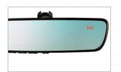
Auto-dimming Mirror with HomeLink.® This upgraded auto-dimming mirror detects glare and darkens automatically to protect your vision while featuring an 8-point digital compass. Three backlit HomeLink® buttons can be programmed to operate most garage doors, security gates, home lighting and more. It can also provide you with the last status of your garage door (open or closed) if programmed to a compatible opener featuring two-way communication.
