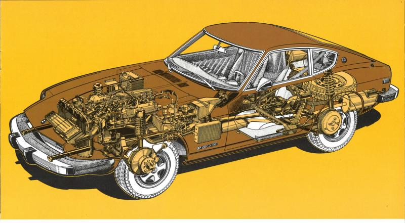
wheel responds individually to road and cornering stress. (Many so-called GTs have a common leaf-spring rear suspension.) Stabilizer bars fore and aft and rack and pinion steering complete the sensitive, sophisticated package.
