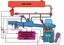
meter exact amounts for all driving conditions. More efficient than carburetors, fuel injection boosts fuel economy and cuts emissions with a lean mixture. Improves performance with a low resistance intake system. Special temperature controls speed cold weather starts.
