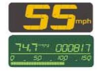
The middle of the Electronic Instrument Display provides a wealth of information, including present speed, the distance the car has traveled, and both current and cumulative fuel economy.
