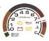
The Insight's Electronic Instrument Display is logical and easy to read: on the left is engine status information, such as rpm and engine coolant temperature.
