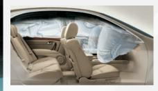
ADVANCED AIRBAG SYSTEM THE RL'S IMPRESSIVE LIST OF PASSIVE SAFETY FEATURES INCLUDES DUAL FRONT AIRBAGS, FRONT SIDE AIRBAGS AND SIDE CURTAIN AIRBAGS. AN ARRAY OF SENSORS MONITOR IMPACT ANGLE AND SEVERITY, AS WELLAS SEAT-BELT USAGE AND THE SIZE AND POSITION OF THE FRONT PASSENGER TO HELP THE AIRBAGS DEPLOY PROPERLY.<sup>®</sup>
