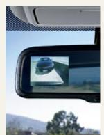
Rearview camera on EX-L models utilizes a portion of the rearview mirror as a full-color camera display when you engage reverse. On Touring models, the image is displayed on the vehicle's navigation screen.
