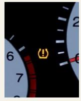
Tire Pressure Monitoring System<sup>9</sup> (TPMS) notifies you with a warning indicator in the information display if air pressure in a specific tire is significantly low. Touring model gives you an individual pressure readout for each tire.
