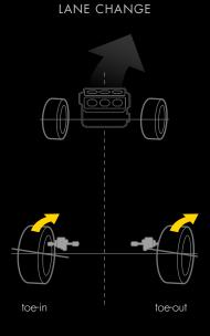
While braking, each rear wheel adjusts inward, increasing stability.
