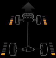
As weight shifts to the rear of the TLX during hard acceleration, the SH-AWD system transfers up to 44% of the power to the rear wheels to take advantage of available traction.
