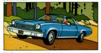
El Camino's new front bumper system Double bumper uses full-width inner and outer bumper system. bars, combined with two hydraulic/ pneumatic cylinders to help provide increased protection.
