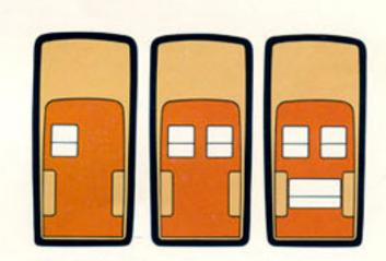
The standard Jimmy is equipped with a bucket-type driver's seat. An auxiliary front passenger bucket seat is also available. Other available seat combinations include twin deep foam front bucket seats with special trim and center console and a three-passenger, full-width rear bench seat. Seat belts are standard for all passenger positions.
