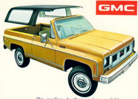
The auxiliary hardtop roof is available with a white or black textured exterior finish. Designed for fast and easy removal, it includes a new tailgate design with manually operated drop glass. Increased side and rear glass areas improve the already broad field of vision. A new accessory roof-mounted luggage carrier is also available.
