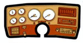
Wraparound cockpit instrument and control cluster design places all gauges, warning lights and controls directly in front of the driver for easy reading and access. Available instruments include: oil pressure gauge, ammeter, coolant temperature gauge and tachometer or clock.
