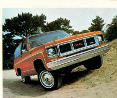
A standard front stabilizer bar; longer, wider front springs; a new extended wheelbase and a tight turning front driving axle gives Jimmy added agility in close off-road driving situations. Two-wheel-drive models continue to present the time proven Independent Front Suspension with new rubber bushings for your driving pleasure.
