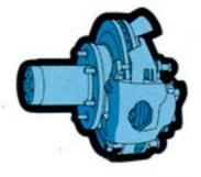
Single-piston caliper type front disc brakes with power assist, road splash shield and rear, finned, aircooled drum brakes are standard.
