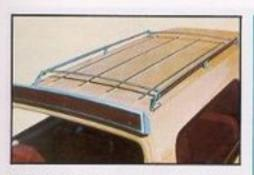
Available as an accessory, a roof rack adds to the smart appearance of your Suburban and gives you even more cargo capacity. The roof rack provides a secure tie-down for extra bulky objects.
