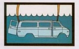
Rally Wagon bodies are electrocoated with rust-resisting primer before painting. Body and doors are completely immersed in a bath of special prime paint, electrically charged to draw the rust-resisting emulsion into corners and crevices. '76 Rally Wagons have additional anticorrosion measures in many critical areas.
