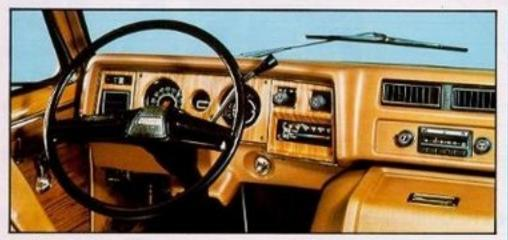
Recessed instrument cluster is grouped for easy viewing. Instrument panel is color-keyed and padded. Control knobs have international symbols for quick identification and are within easy reach of the driver. Optional air conditioning is shown.
