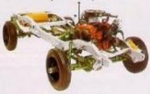
equipped with an inter-axle differential that balances the speed variations between front and rear axles and locks manually into conventional four-wheel-drive for poor traction situations like loose sand or slippery snow. A front stabilizer bar, tapered front leaf springs, and power brakes are standard.
