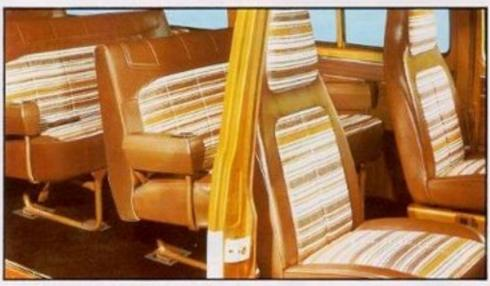
Rally STX models provide floor length carpeting, including front and rear wheel housings, woodgrained vinyl trim on door and side trim panels, a choice of striped nylon and vinyl or all-vinyl seat trim and highbacked bucket driver and front passenger seats. Standard and Custom Rally Wagon model features include good-looking all-vinyl seat trim, complete floor insulation and floor length rubber mats.
