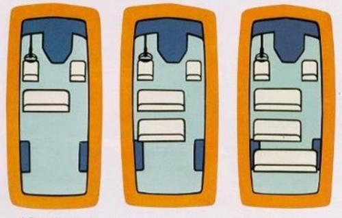
A Rally Wagon comes with driver and front passenger bucket seats plus a full-width seat. A second full-width seat increases capacity to eight. And a third seat, only optional on 1-ton units, can bring total accommodation all the way up to twelve people.
