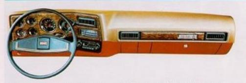
An efficient wraparound instrument panel is standard. The High Sierra option for Jimmy includes simulated woodgrain accents and full instrumentation with gauges for oil pressure, temperature and voltage. You can also add a clock or tachometer.
