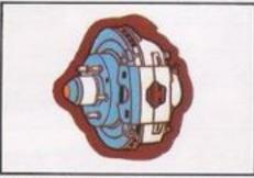
Front brakes are discs for added resistance to heat, water and fading. Cast iron-steel rear brake drums are finned for efficient cooling. Power assist is standard for both the front disc brakes and the rear drums and specially selected for heavy-duty operation.
