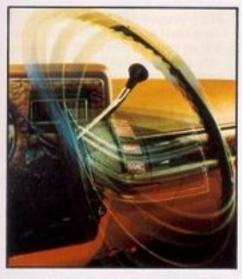
The optional tilt steering column adjusts to six different positions so you can choose your most comfortable angle. An adjustable column also helps make getting in and out of your Suburban easier.
