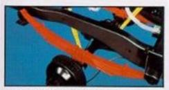
Two stage leaf spring rear suspension is standard. Staggered-mounted shock absorbers offset on each side of the axle help dampen out brake thrusts and power hop.
