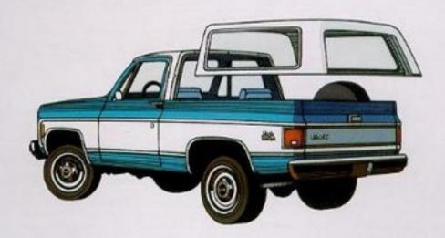
New half-cab Jimmy design incorporates integral steel roof and full doors for front compartment, removable fibreglass roof for rear compartment section. Tailgate is designed with manually-operated dropglass.
