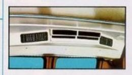
This unit, located in the rear, cools and recirculates the inside air pre-cooled by the optional front air conditioner.
