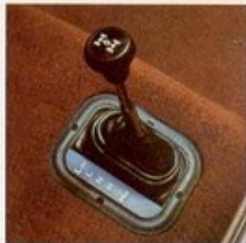
drive. "H-LOC" locks out the inter-axle and connects both front and rear axles while operating in direct drive. It is used when low traction surfaces could cause wheel slippage. With Full-Time four-wheel drive, included in conjunction with available automatic transmission and V8 engine, you enjoy balanced driving power and traction effort at all four wheels. GMC
