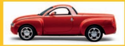
The retractable roof consists of two stamped steel panels and a deep-tinted fixed backglass. Triple weather seals provide the added protection needed for the Canadian climate.
