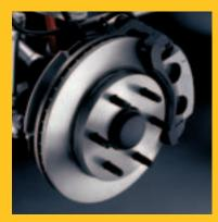
The standard 4-wheel disc braking system includes ABS and dynamic rear proportioning (DRP).
