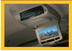
A rear-seat, fold-down 178 mm (7 in.) colour LCD monitor, audio/video input jacks for camcorder playback and video games, two wireless infrared headphones, and a remote control unit is available on Tahoe and Suburban.
