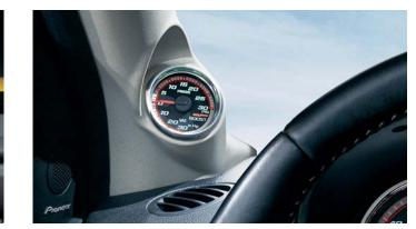
SS Turbocharged models include an A-pillar-mounted boost gauge.
