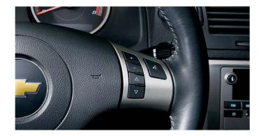
Steering wheel-mounted audio and cruise controls.
