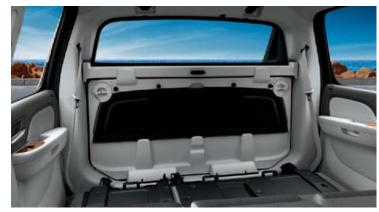
**2** To begin converting Avalanche from an SUV to a pickup, simply lower the 60/40 split-folding bench seat. You can also stow the rear window inside the Midgate.
