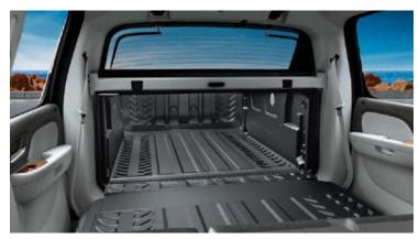
**3** To utilize the full length of the cargo box, just lower the Midgate for a completely secured cargo area (when the three-piece cargo cover and rear window are in place).
