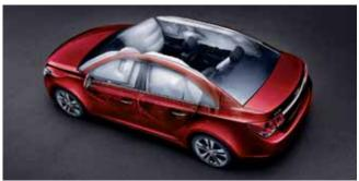
**Ten Air Bags:** Standard on every Cruze, including frontal, front side-impact, roof rail-mounted head-curtain side-impact with rollover capability, outboard rear side-impact, and new knee air bags.
