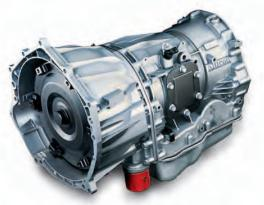
$\label{thm:continuous} \textbf{HARNESSING THE POWER} \ of the \ available \ Duramax \ 6.6L \ Turbo-Diesel \ V8 \ engine is the renowned \ Allison \ 6-speed \ automatic \ transmission.$
