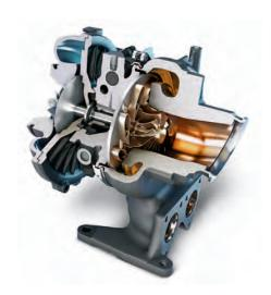
**EXHAUST BRAKE SYSTEM** The diesel exhaust brake system on the available Duramax 6.6L Turbo-Diesel V8 engine works in conjunction with the Tow/Haul mode and auto grade braking features. After adjusting for the load and grade, a variable vane geometry turbo creates back pressure to slow the vehicle down, help reduce brake use and conserve your brake pads.
