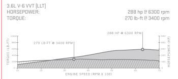
VARIABLE VALVE TIMING (VVT) This gives you the power of a highperformance engine with the low-speed response you need for situations such as trailering or climbing steep inclines. This technology constantly monitors and changes how the valves open and close to give you near-peak levels of torque across the entire range of engine speeds.
