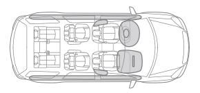
HEAD CURTAIN SIDE-IMPACT AIR BAGS<sup>11</sup> These air bags unfurl from the roof rail like a protective curtain for outboard passengers and can be activated by either rollover sensors or side-impact sensors.
