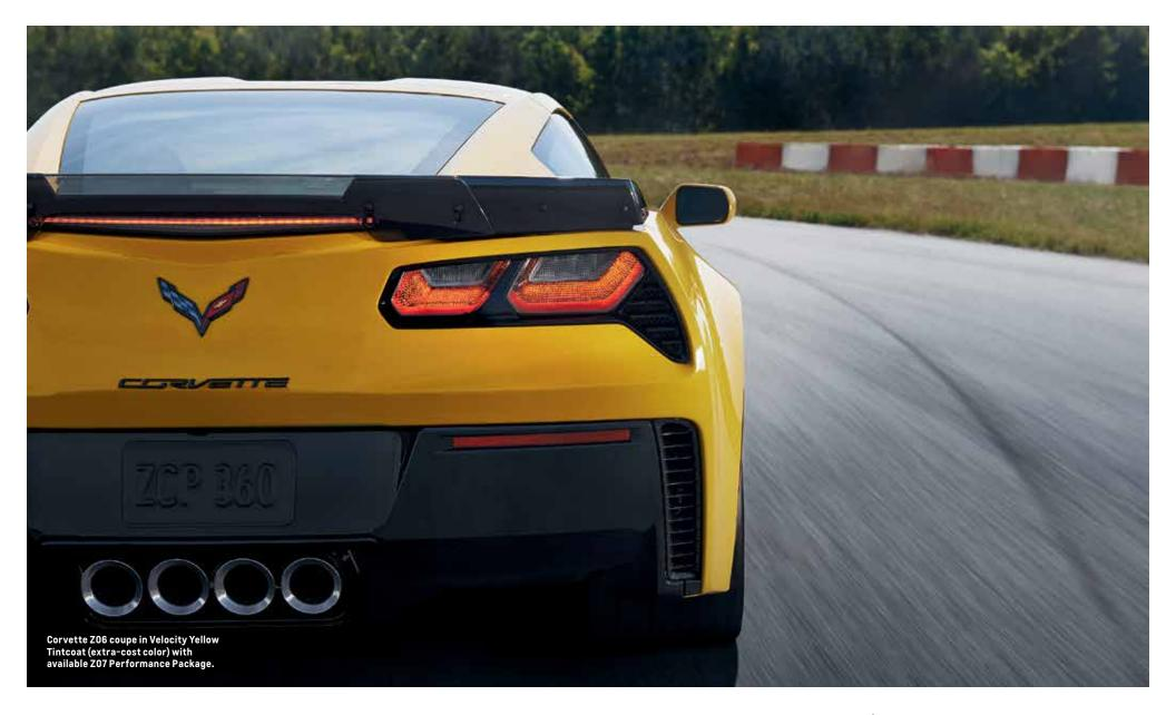
650-HP SUPERCAR. Z06 is powered by the LT4 6.2L supercharged aluminum V8 delivering 650 horsepower and 650 lb.-ft. of torque. It incorporates an efficient next-generation supercharger, as well as a dry-sump oil system and titanium intake valves and connecting rods for reduced mass.
