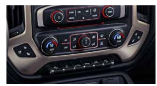
**CLIMATE CONTROL** Automatic dual-zone climate control with individual settings for the driver and front-seat passenger is standard on SLT and Denali and available on SLE.
