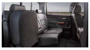
**REAR-SEAT ACCESS** Rear-seat comfort is the result of 40.9" of leg room on Crew Cabs. And getting into and out of the second row in the Double Cab is easy, thanks to forward-hinged rear doors.
