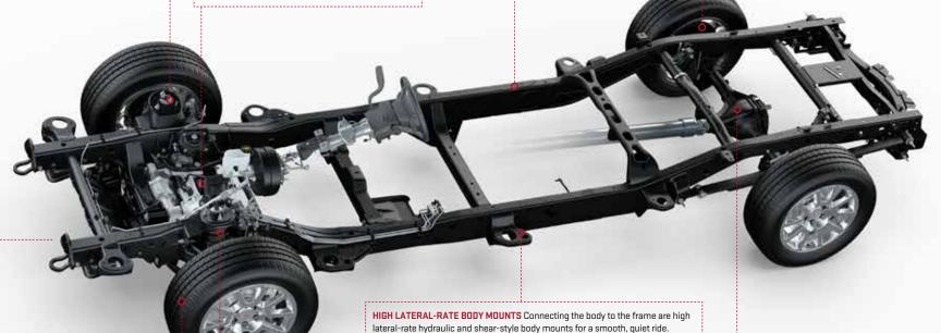
**COIL-OVER-SHOCK FRONT SUSPENSION** This fully independent system is precisely tuned for improved handling.
