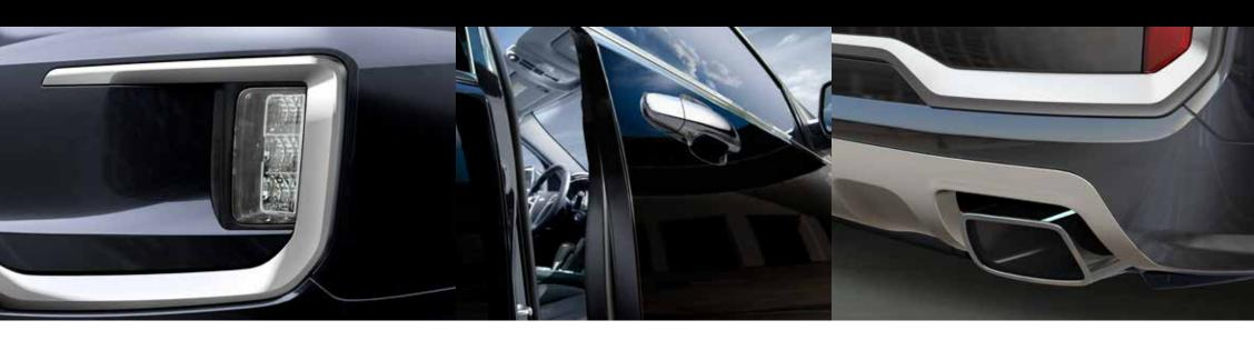
INTEGRATED LED DAYTIME RUNNING LAMPS For daytime illumination, Terrain offers LED daytime running lamps for excellent visibility and durability.
