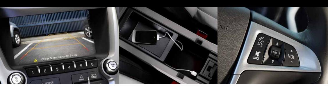
REAR VISION CAMERA SYSTEM It displays a real-time image with grid lines in the color touch-screen while in reverse, making it easier and safer when backing up. Shown with available Rear Cross Traffic Alert.
