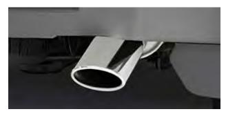
**EXHAUST TIP** This stainless-steel dual-wall, angle-cut exhaust tip adds a sporty appearance to the exterior of your Yukon. Use only on GM's Original Equipment exhaust system.
