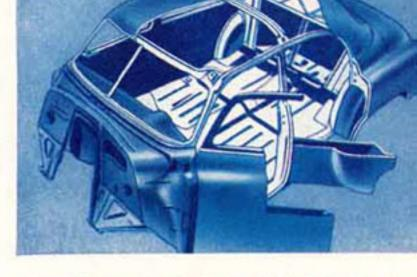
The body construction protects you with a solid steel "cradle" of great strength—steel welded to steel all about you. Even the instrument panel is welded into the body structure for greater strength and safety.
