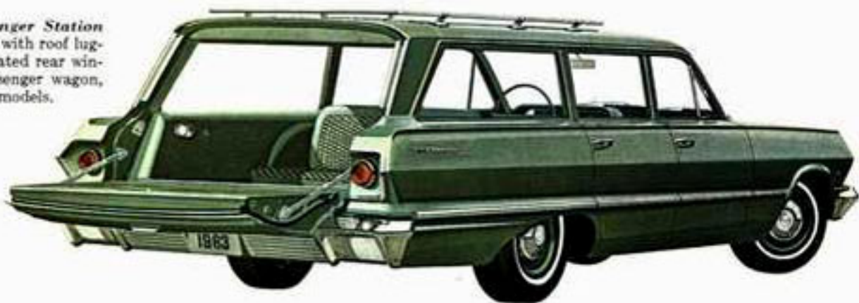
Biscayne 4-Door 6-Passenger Station Wagon in Tuxedo Black. Huge tailgate opening in wagons measures 30.5 inches high and 56.3 inches wide at the floor.
