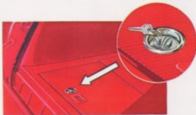
REAR FLOOR COMPARTMENT LOCK —For the storage compartment in the floor of the luggage compartment.
