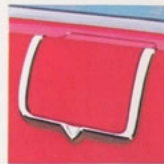
GASOLINE FILLER DOOR GUARD —Protects paint from being marred and scratched by the gasoline pump nozzle.
