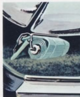
SEAT BELT RETRACTORS —Keeps belts from accidentally hanging out the door and being damaged by closing the door on the belt. Keeps the belt clean and rolled into a neat roll at the floor level near the front seat.
