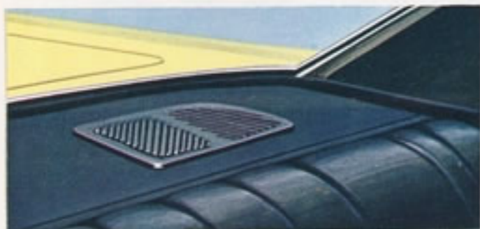
REAR WINDOW DEFROSTER —Directs warm forced air over the window to clear the glass of fog, ice and snow. Also helps air conditioner circulate cool air in rear compartment.
