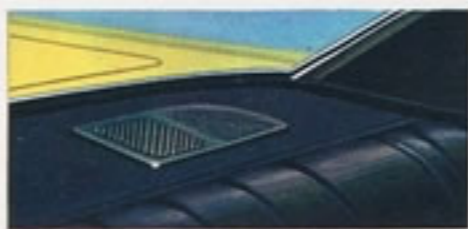
REAR WINDOW DEFROSTER —Directs a stream of warm air over the rear window to help reduce fog, ice and snow from the window.
