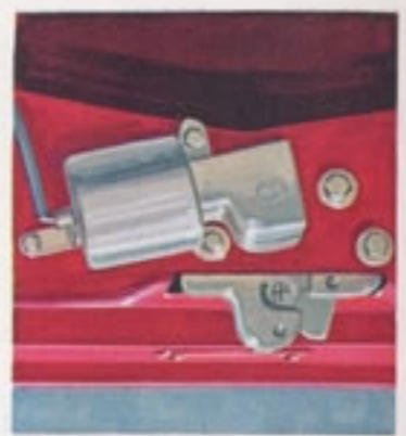
AUTOMATIC TRUNK OPENER —A control valve located in the glove compartment automatically opens the trunk lid.
