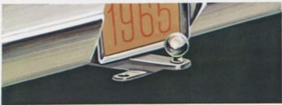
TRAILER HITCH —A stable hitch ideal for light utility or boat trailers, designed to handle a 2000 pound load with a 200 pound vertical tongue load. A trailer wiring harness is also available.
