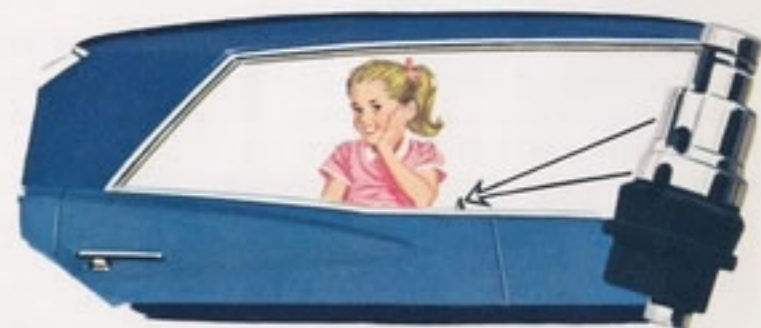
DOOR SAFETY LOCKS —When door locks are depressed, the rear doors can not be opened without a key-like object to lift the button. Can be used on all doors.
