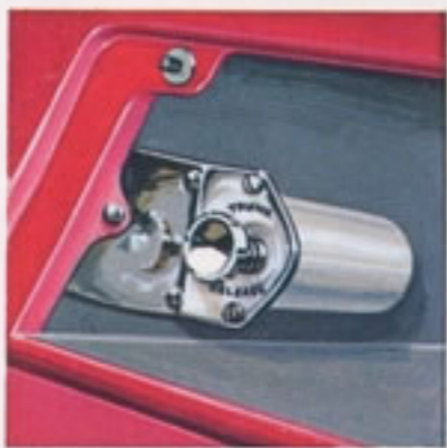
AUTOMATIC TRUNK OPENER —A control valve located in the glove compartment automatically opens the trunk lid.
