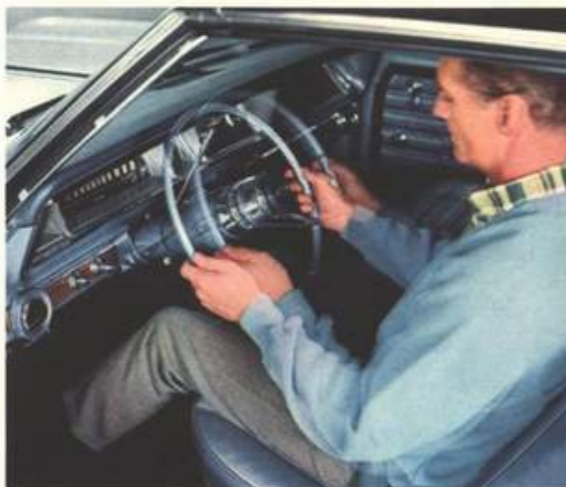
Top: COMFORTRON AUTOMATIC HEATING AND COOLING lets you set the dial for the comfort level you want; then it automatically keeps your Chevrolet interior warm in the chilly season, air conditioned and dehumidified in hot weather.
