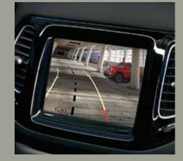
WITH DYNAMIC GRID LINES BACK OUT SAFELY WITH GRACE. THIS SYSTEM HELPS BRING PREVIOUSLY HIDDEN REAR OBJECTS TO YOUR ATTENTION, EITHER ON-SCREEN OR WITH AN AUDIBLE WARNING, IN GOOD TIME TO REACT. STANDARD.
