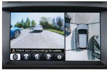
All-Around Views In addition to its rearview camera, Santa Fe's Multi-view Camera displays an overhead view to help you see the area all around your vehicle. The touchscreen display's split screen also allows you to view navigation maps and music apps simultaneously. Welcome to multitasking at its most effortless.
