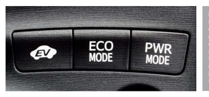
**EV/ECO/POWER MODES** Prius has different modes for different types of driving. Eco mode helps maximize fuel economy. EV mode<sup>1</sup> drives solely on battery power for up to one-half mile under certain conditions. And Power mode increases gas pedal sensitivity for additional get-up-and-go.
