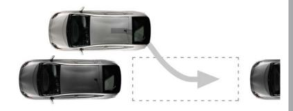
**ADVANCED PARKING GUIDANCE SYSTEM (APGS)**<sup>1, 2</sup> Parallel parking made easy: Press the available Advanced Parking Guidance System (APGS) button when approaching the spot and an image of the parking spot appears on the navigation screen, with a box indicating the final position of the vehicle. Once the driver approves the position, Prius virtually parks itself, only requiring soft braking by the driver to stop the vehicle in the desired parking spot.
