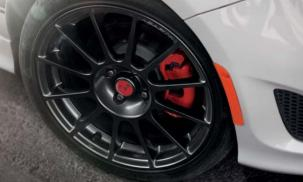
Track-ready performance means the ability to slow things down in a hurry, as well. Abarth braking performance is top-notch with large-diameter ventilated front rotors, Rosso (Red) single-piston front and rear brake calipers, and semimetallic brake linings.
