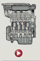
THE I.4L I6V MULTIAIR ENGINE This exclusive FIAT technology, a decade in the making, utilizes electrohydraulic valves for more dynamic and direct control of air and combustion. Power is improved up to 10 percent, torque goes up 15 percent and fuel efficiency has a 10 percent advantage over conventional naturally aspirated engines. Emissions, in turn, are cut an impressive 10 percent. The MultiAir engine boasts 101 horsepower at 6,500 rpm and 98 lb-ft of torque at 4,000 rpm.
