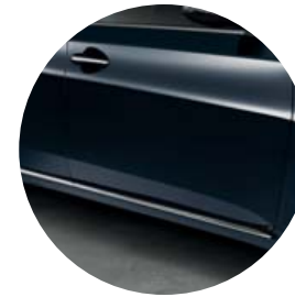
Lower door molding
