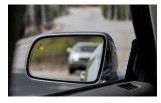
BLIS® (BLIND SPOT INFORMATION SYSTEM) WITH CROSS-TRAFFIC ALERT 1,2 - Some vehicles may be out of your line of sight, but they can be detected by this technology. It warns you if it detects a vehicle in your blind spots while driving forward, or approaching from the sides while in Reverse.
