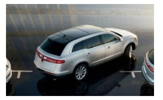
**ACTIVE PARK ASSIST**<sup>1,2</sup> – For help parallel parking, simply activate this system. It uses ultrasonic sensors to help you locate an appropriate space, then steers MKT into it. All you do is follow on-screen prompts and control the shifter, brake and accelerator pedals. For additional guidance during parking maneuvers, a Reverse Sensing System<sup>2</sup> and rear view camera<sup>2</sup> are standard on every MKT.
