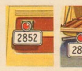
TAIL LIGHT and license-plate holder swivels to position shown above at right when tailgate is left down to haul bulky objects.
