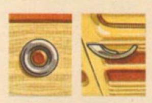
DOOR LATCHES are finest trigger-andbutton type. Exterior handle is closed at both ends-prevents torn pockets.
