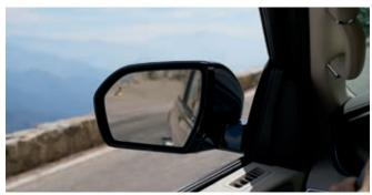
BLIS® (BLIND SPOT INFORMATION SYSTEM) WITH TRAILER COVERAGE!— Some vehicles may be out of your line of sight, but they can be detected by this technology. It warns you if it detects a vehicle in your blind spots while driving forward, or approaching from the sides while in Reverse. The range of coverage can also be extended to include a conventional trailer, once it's been programmed into the system.
