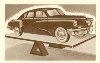
Precision Balance - The unique Tucker design distributes weight to give maximum safety, maximum power transmission, feather-light steering and driving control, and-for the first time-insures complete four-wheel traction in braking. Only a rear engine car can achieve this precision balance for years the goal of all automotive engineers.
