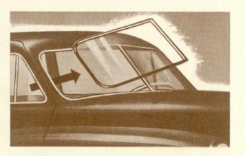
Safety Windshield—Laminated safety glass is mounted in sponge rubber fastening so that a hard blow from within will eject it in one piece. Thus, greatest collision hazardlacerations or fractured skull from striking windshield-is entirely eliminated. Windows are armor-plate glass which disintegrates without cutting edges or slivers.
