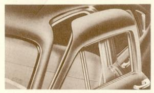
Roof Top doors are another exclusive Tucker comfort feature. The doors are curved at the top so that they become part of the roof itself. As a result, getting in and out of the Tucker is a new experience in ease and comfort. Even from a high curb, exit or entrance is made without the usual jack-knife bend.
