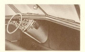
Crash Board Cowl and Safety Chamber—Conventional instrument panel is replaced by attractive sponge rubber crash board cowl. Instruments in steering column. Under cowl is spacious safety chamber, protected by steel bulkheads, which driver and front seat occupants can drop into, in a split second, in case of impending collision.
