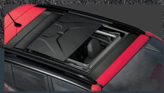
The My Sky® power retraction operates like a traditional sunroof, allowing fore and aft ventilation with the front panel. Press the button for quick and easy rooftop ventilation.
