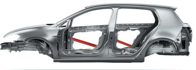
Front and rear crumple zones help absorb crash energy, while a rigid safety cage helps deflect it away from the driver and passengers.
