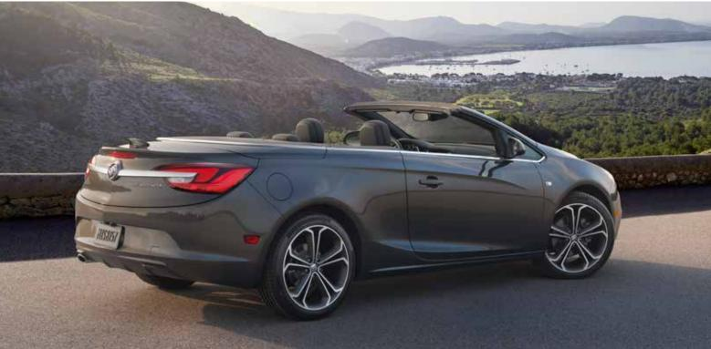
Cascada's convertible top automatically retracts. The rear decklid opens, and the top neatly folds and stows under a hard tonneau cover. Easy activation lowers the top in just 17 seconds, and puts the top back up in only 19 seconds, at speeds of up to 31 mph. Want the top up? It's easy to see why. With available top colors Ebony, Malbec and Sweet Mocha, Cascada is that rare convertible that's as stylish with the top up as it is down.
