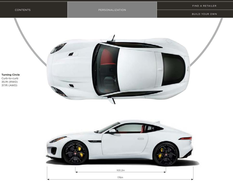
Dimensions were measured with vehicle at unladen weight. Figures shown are for F-TYPE R. See pages 110-111 for full details on Technical Specifications.
